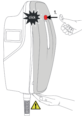
Fig. 19: Attach front cover (example) - 1
